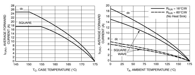
Figure 3. Current Derating, Case, Per Leg
