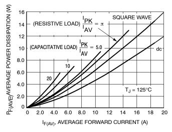
Figure 5. Forward Power Dissipation
